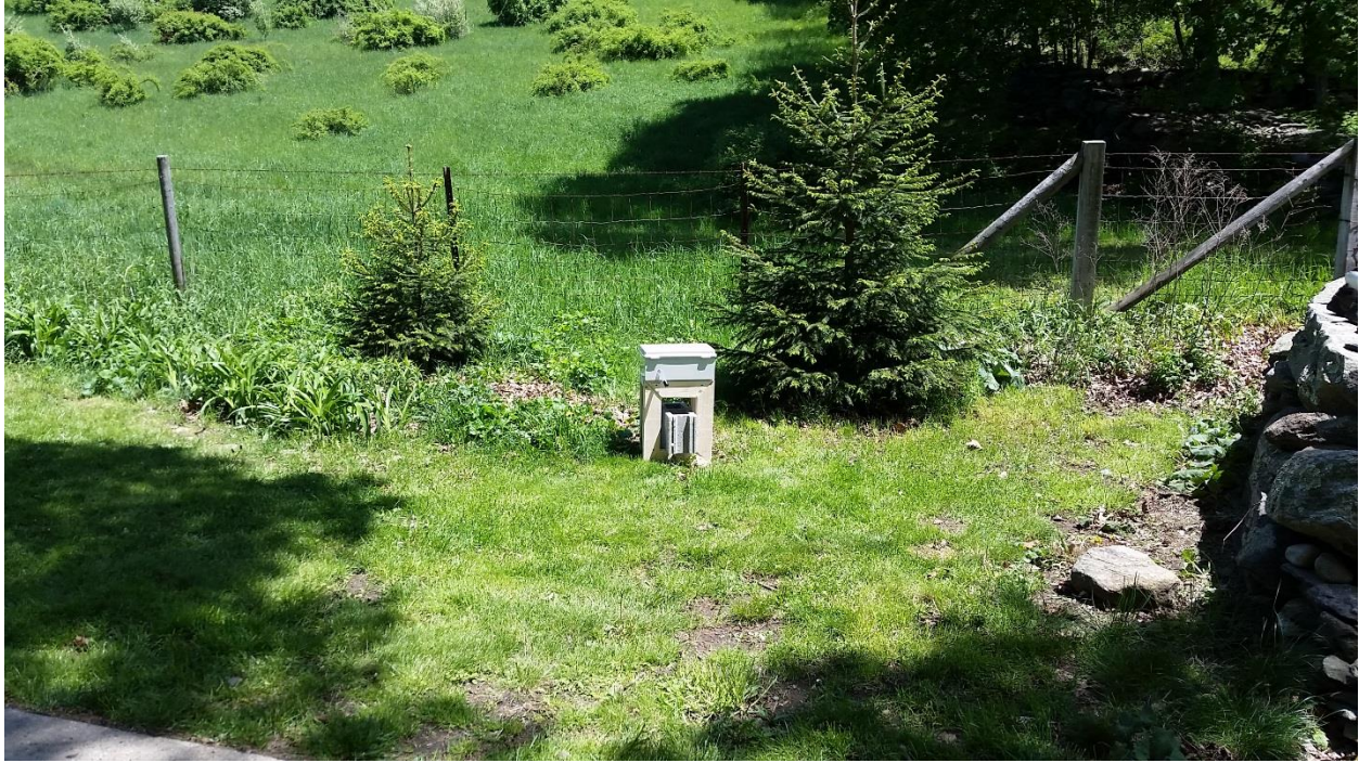
Figure 7. Particulate matter monitoring enclosure at the SVSF. A cinder block was used to secure it in place.
